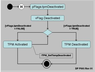
Figure 7:d - Activated and Deactivated States
